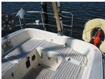
The teak surfaces on this 8 year old HR34 were treated every autumn with Boracol 10Rh. Halberg Rassy recommend Boracol 10Rh for teak surfaces on their boats.
