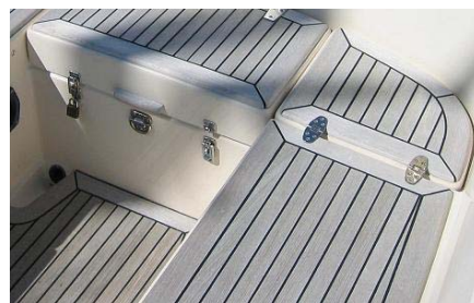
The teak surfaces on this 8 year old HR34 were treated every autumn with Boracol 10Rh. Halberg Rassy recommend Boracol 10Rh for teak surfaces on their boats.
